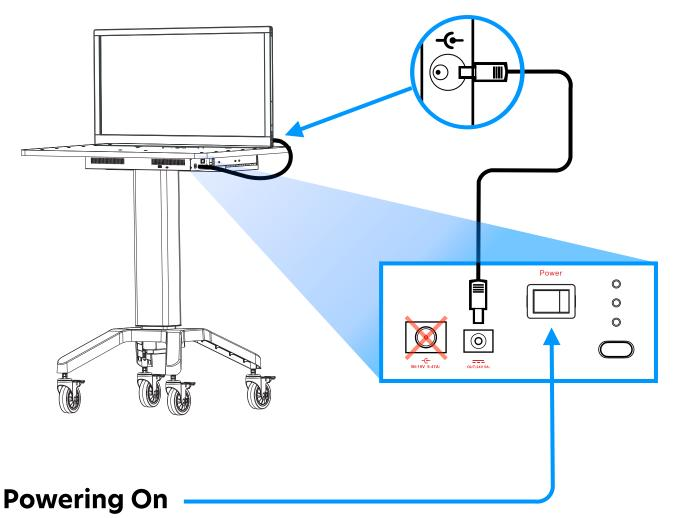
To power on (and off) the eGlass Station battery, activate the **Power Switch** located on the left underside of the **Podium Surface**.
